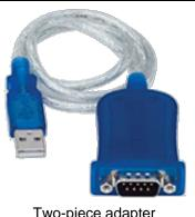
Two-piece adapter (serial cable not shown)
